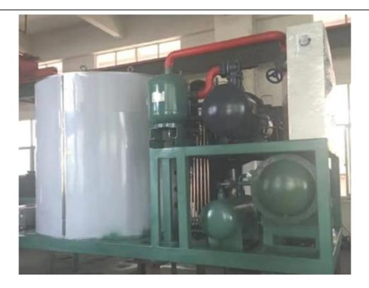
The unit's piping is meticulously designed and expertly welded, ensuring stability, durability, and a leak-free, extended service life. High-temperature pipelines are clearly marked with red paint for safety.
