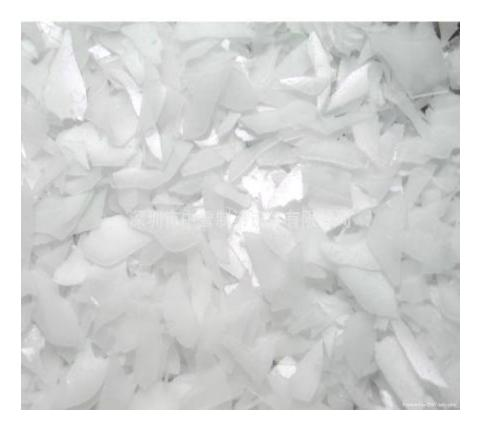
Flake ice is produced by ice machines and as produced isdelivered by a roots style blower up to 150 metres from the ice machine position where it can be blown into stockpiles or delivered to a patented Bucceri B4 snow maker that converts the ice into fresh snow or if the temperature is low enough uses the ice as a nucleating agent for atomised water to make large amounts of snow. The snow produced can be up to 20 times the ice quantity if the conditions are right.
