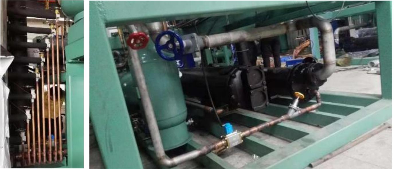
Maintenance is simplified with shut-off valves strategically placed at both ends of each accessory pipeline.
