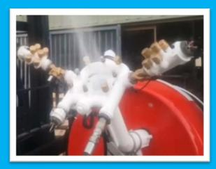
Atomised water usage shown below at -3 degrees Celsius (7 Degrees Fahrenheit) Wet Bulb assume an Ice Nucleation production of 2.5 litres per minute 0.625 Gallons per minute.
